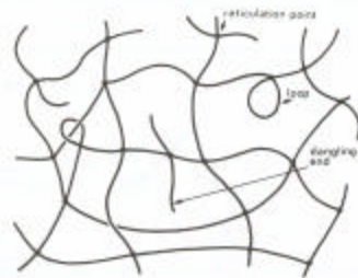
Figure 5.8 Schematic of a cross-linked polymer network. (Reprinted from Flory-Ciffo di Gennaro, Scaling Concepts in Polymer Physics , Copyright © 1979, by Cornell University. Used by permission of the publisher, Cornell University Press.)
